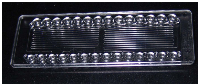
Figure 2 Image of a CrystalCard showing the two microcapillary channels.
